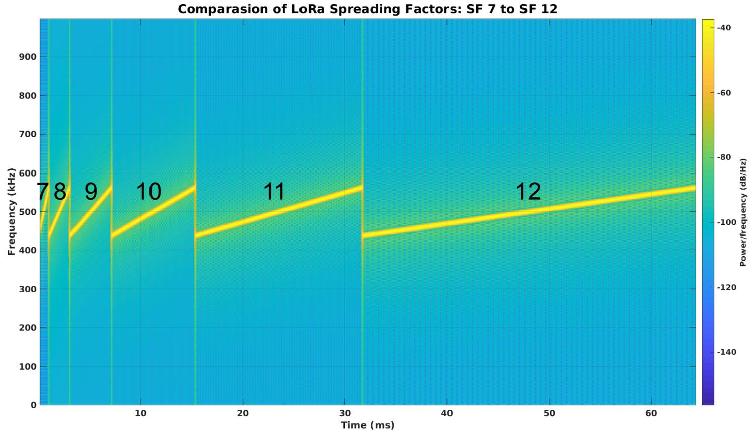
For a given bandwidth : Higher SF = Higher time on air, Lower Packet Error Rate, Longer Coverage (but Lower Symbol rate)
